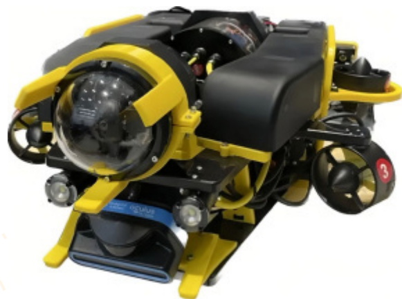
ORVIS 自主水下載具 The ORVIS Autonomous Underwater Vehicle
